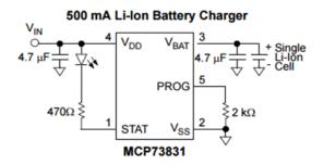
This circuit worked right away and was less complicated than our first design. Ultimately, this will only work with a single cell Li-Ion battery, so we couldn't use it in our final board design.
